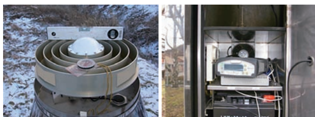
Fig.5 Antenna being renewed (left) and GNSS receiver (right)
