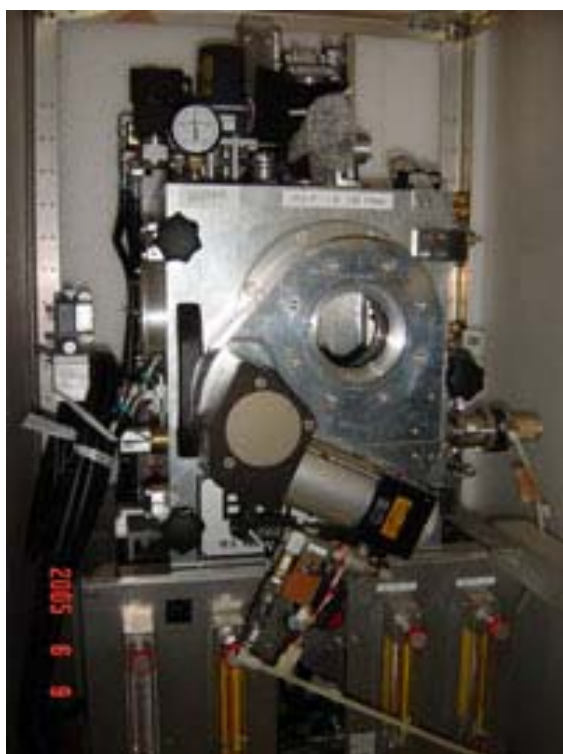
Fig. 1 Electromagnetic levitator (PFLEX) for use in surface tension measurement in an ambient atmosphere with various oxygen partial pressures during a parabolic flight of a jet plane.
