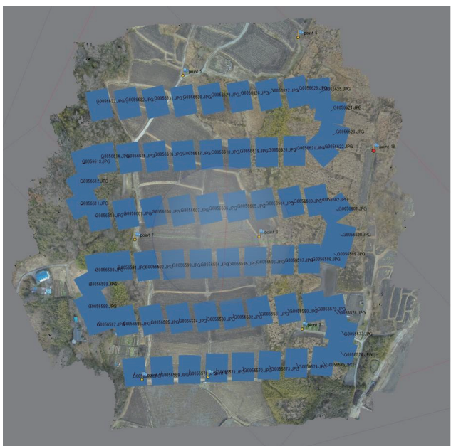
Fig. 73 Aerial photos taken from 100 m above the ground with GoProHero3 (medium FOV) at a foot of Mt.Hokyo. Each photo overlaps 80 % to the adjacent photos.
