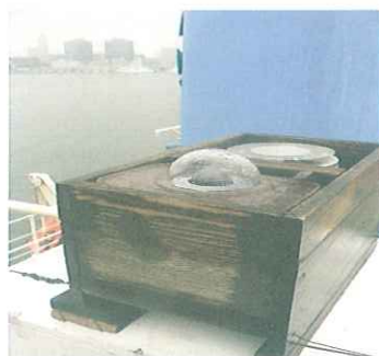
Fig. 1 All sky camera (front) and field mill (behind) set up on the upper deck of the R/V Hakuho Maru.
