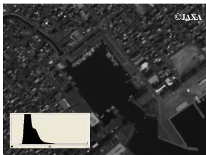
Fig. 8 Image without radiometric correction, inset shows the histogram (Sensor's sensitivity: Gain 2)
