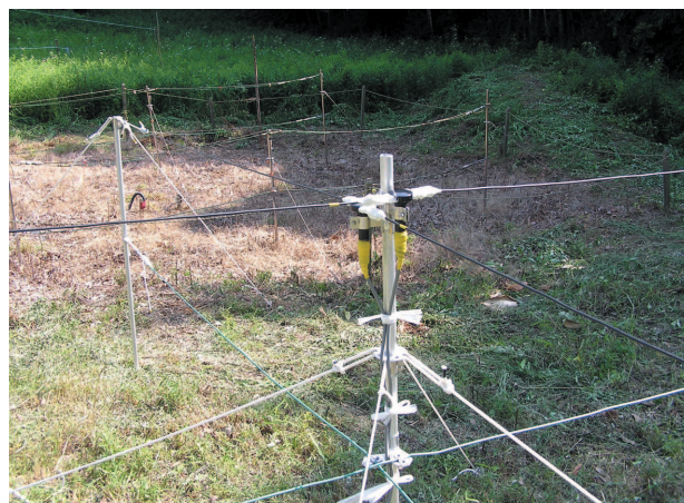
Fig.7 Polarization riometer antenna installed at Kakioka Geomagnetic Observatory
