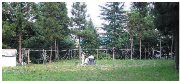
Fig.3 Testing of Imaging riometer installed at Takushoku University Campus
