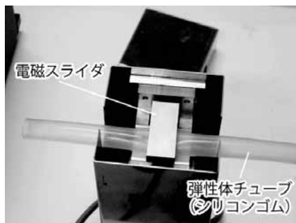
Fig. 8 Prototype electrical control type speech valve
