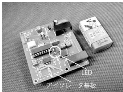
Fig. 5 Miniaturized control circuit with one-chip microcomputer
