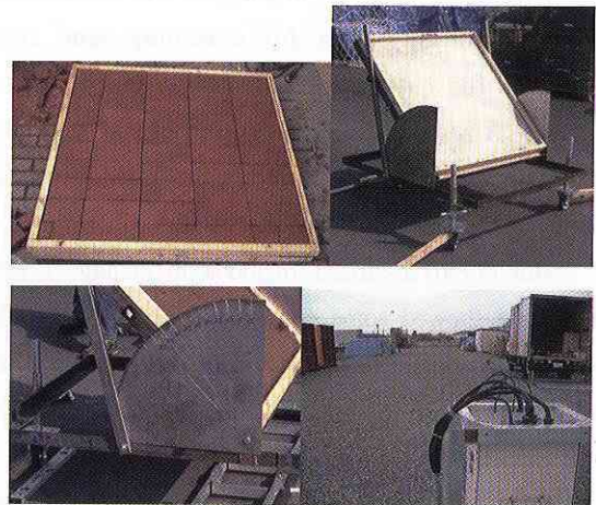
Fig. 1 Equipment for on the ground survey. The brick target (top left) and the holder with the target (top right). The target is 1m square. The holder has protractors on both sides (bottom left). Looking at the target from near the laser scanner (top right).
