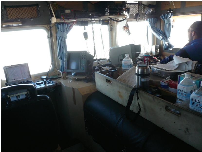
図 13 雪上車の前部を占める船舶航行用レーダ（左側）と船舶航行用 GPS（右側） Fig. 13. Displays from the Marine Navigation GPS and Marine Navigation radar, occupying the front inner part of the tracked vehicle.
