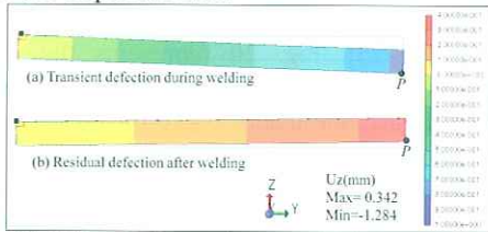
Fig. 10. Welding deformation mode during welding and cooling by ACEXP method
