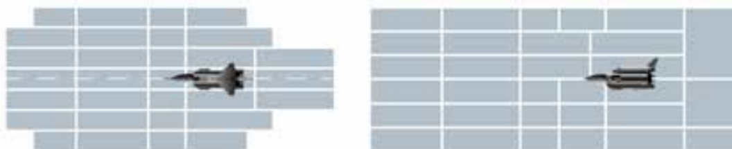
Figure 1. Arrangement of the T-128 perforated panels and the location of the model in the test section No 1
