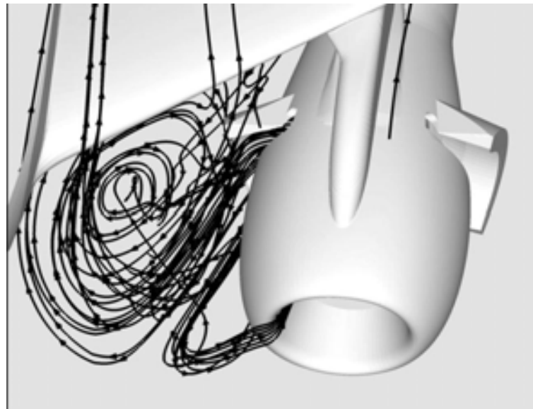
Figure 17. 3D flow reconstruction of reingestion
