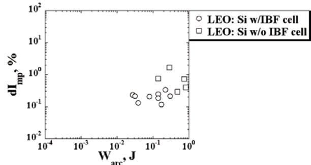
Fig.5 Relationship between  $dI_{mp}$  and  $W_{arc}$  on a Si w/IBF cell and on a Si w/o IBF cell
