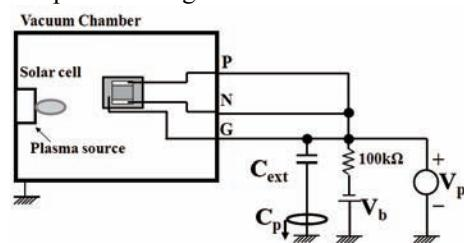
Fig.3 Discharge circuit
