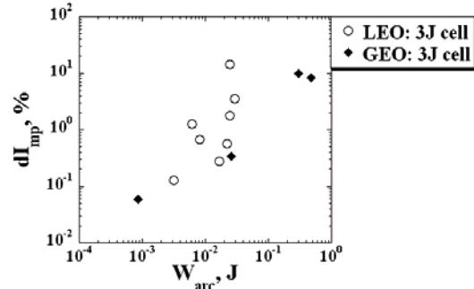
Fig.4 Relationship between  $dI_{mp}$  and  $W_{arc}$  on a 3J cell
