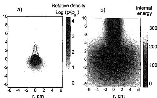
Fig. 1: Distribution of relative density (a) and dimensionless internal energy (b) around a 1 cm body at 100 km altitude
