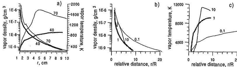
Fig. 2: Dependence of vapor cloud parameters at 100 km altitude (a) on velocity  $V$  (40 km/s and 70 km/s, given at the curves,  $R=1$  cm); (b,c) on meteoroid size  $R$  (0.1, 1 and 10 cm, marked at the curves,  $V=40$  km/s).
