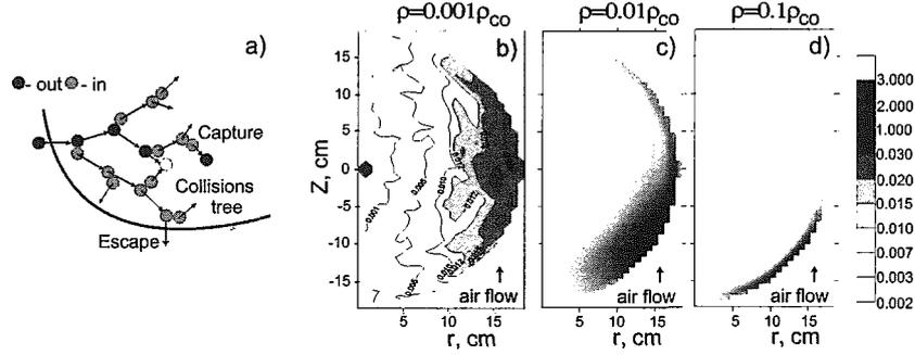
Fig. 3: a) schematic picture of particles trajectories; (b, c, d) absorbed energy spatial distribution in vapor cloud ( $\rho_{co}=10^{-5}$  g/cm<sup>3</sup>)
